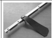
Positioning jigs for cutting oblong plates of sheet metal parts.
