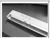
Graduated measuring bar for selecting the correct Jig 1.1
